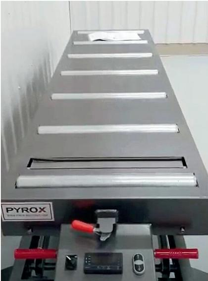
**New loading table with built-in scale.**
